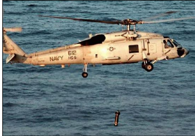
Figure H-5: Helicopter Deploys Dipping Sonar
